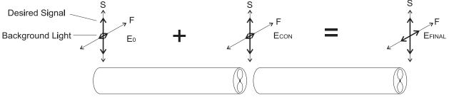
Figure 4: Degradation of Polarization at a Connection
