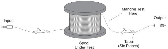
Figure 5: Preparation of A Fiber Spool For Measurement
