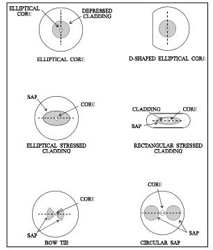
Figure 2: Examples of polarization preserving fiber core structures.
