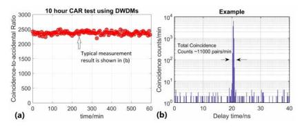
Fig. 3. (a) Coincidence-to-accidental ratio(CAR) in 10 hours using a DWDM filters set with effective bandwidth of 0.85nm, under a pump power of 7.5mW. (b) A typical coincidence example of 1min measurement histogram is randomly selected from (a). It demonstrates around  $1.1 \times 10^4$  pairs/min coincidence counts with around 3dB of losses after the output and 20% detection efficiency at single photon detectors.
