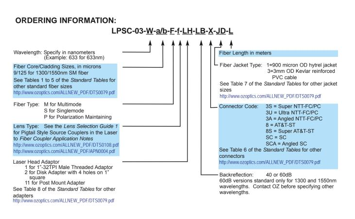
Note: Add "-ER=30" or "-ER=25" to the part number for 30dB or 25dB extinction ratios (For 1300nm and 1550nm only). Add "-BL" to the part number if a manually adjustable attenuator is to be added.
