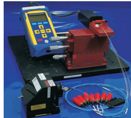
ER-Measurement Test System for V-Groove (Manual Type)
