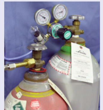
CO 2 & N 2 Cylinders, typical gas supply (USA) connection shown
