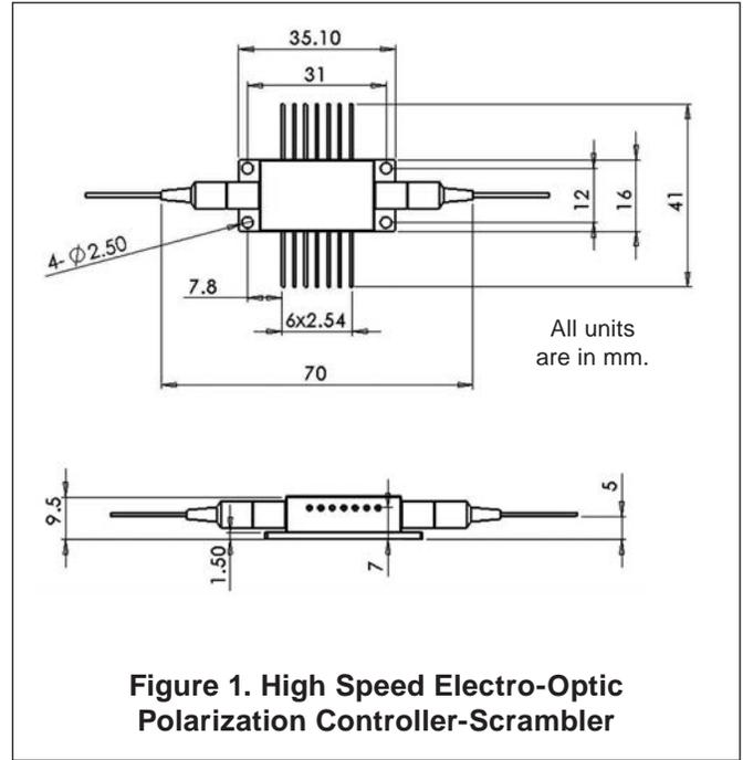
**Figure 1. High Speed Electro-Optic Polarization Controller-Scrambler**
