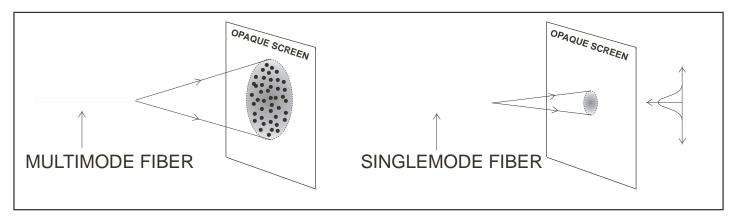
The output from a singlemode fiber (SM) shows a nice, smooth gaussian profile as shown. Singlemode fiber does not maintain polarization under stress such as bending; for that you need polarization maintaining (PM) fiber. PM fiber is also singlemode.
