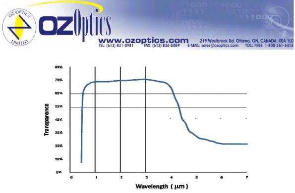
Figure 5. Optical transmission spectrum of EEO crystal wafer with a thickness of 2 mm from 300~7000 nm.
