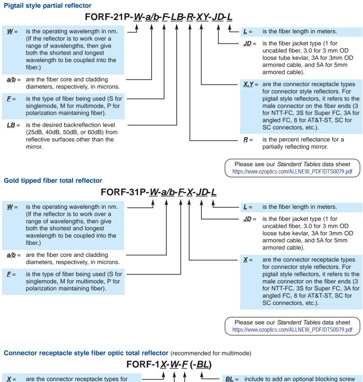
are the connector receptacle types for connector style reflectors. For pigtail style reflectors, it refers to the male connector on the fiber ends (3 for NTT-FC, 3S for Super FC, 3A for angled FC, 8 for AT&T-ST, SC for SC connectors, etc.).
