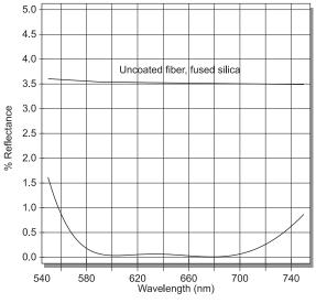
Figure 5: Antireflection coating for 590-690 nm
