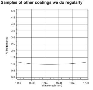
Figure 9: Tap coating, 1% reflectance for 1500-1650 nm
