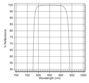
Figure 12: High reflector for 850 nm, normal incidence, R> 99.5%
