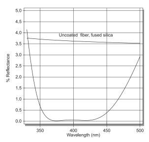
Figure 7: Antireflection coating for 380-430 nm.
