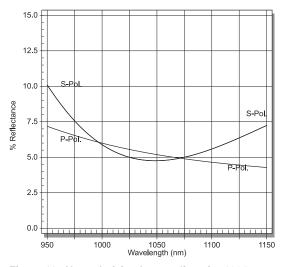
Figure 11: Nonpolarizing beamsplitter for 1064 nm, R/T= 5/95 %, AOI= 45 deg.
