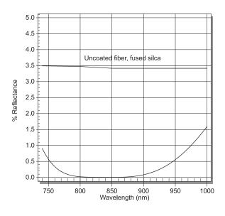
Figure 4: Antireflection coating for 790-890 nm, diode laser applications
