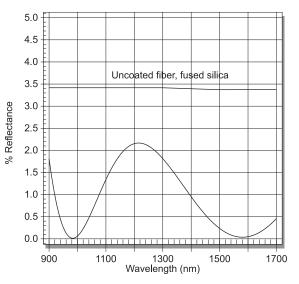
Figure 8: Dual band AR coating for 980 nm and 1550 nm.
