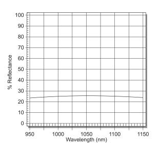
Figure 10: Beamsplitter for 1000-1100 nm, AOI=45 deg. R/T=25/75 %, random polarization
